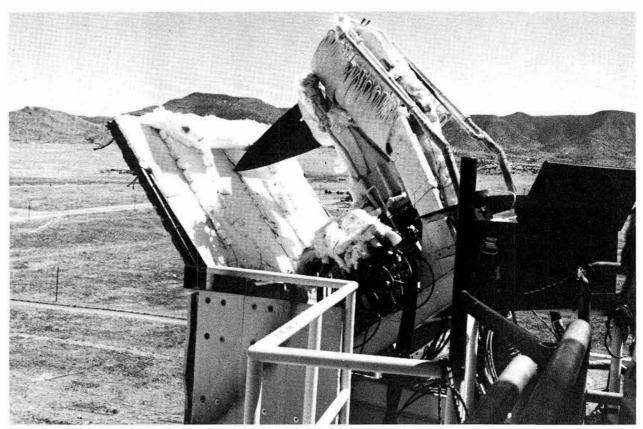
MISSILE RADOME (the black, pointed object) mounted on the Power Tower, ready to be subjected to concentrated sunlight from the heliostats. Test results have led to new radome designs that will minimize radar signal distortion from atmospheric heating.
